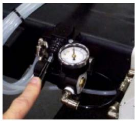
Lever in Down position. Loosen Collet—Relieves the tension on Collet allowing removal of part.
