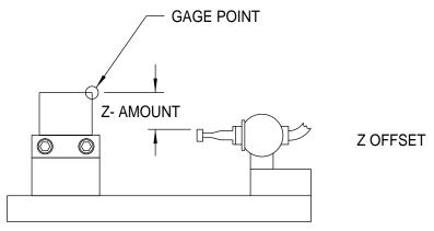
Figure 15-7 Z Fixture Offsets
