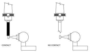
Figure 15-24 Tool Breakage Detection
