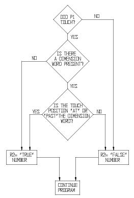
Figure 15-25 Touch Check, Position Check
