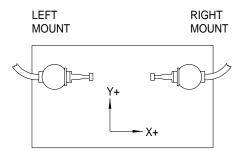
Figure 15-5 Probe Mounting Positions
