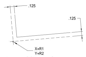
Figure 15-19 CNC Movement to Corner
