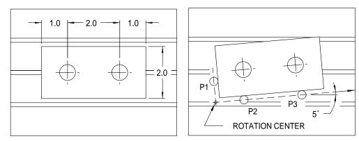
Figure 15-18 Sample Program to Drill Two Holes in a Part
