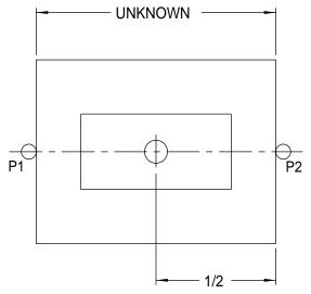
Figure 15-22 Part with Unknown Width
