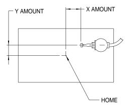
Figure 15-6 Probe Fixture Offset Number
