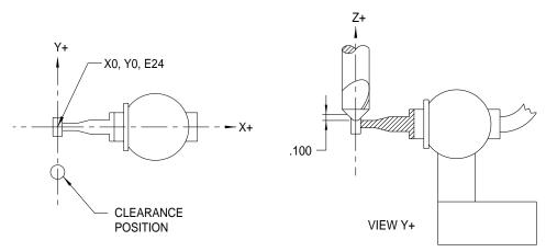
Figure 15-11 Clearance Position & Touch Probe Selection
