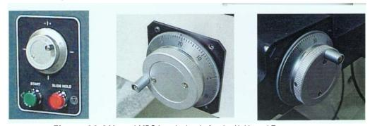
Figure 22-2 Manual MPG hand wheels for the X, Y, and Z axes
