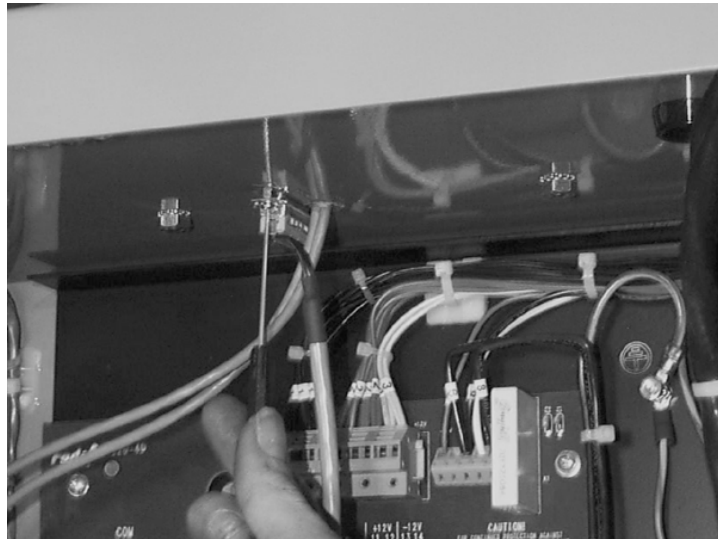
Figure 11-101 Plug 15 Pin Connector into Scale Box Connector
