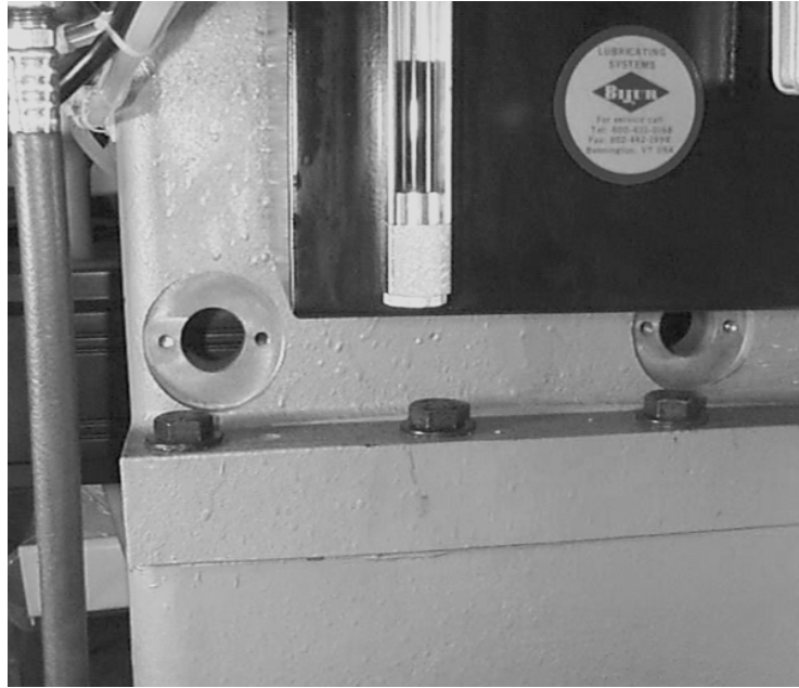
Figure 11-45 Insert Mounts into Openings at Bottom of Column
