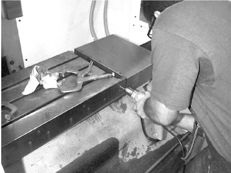
Figure 11-9 Counter Sink Holes
