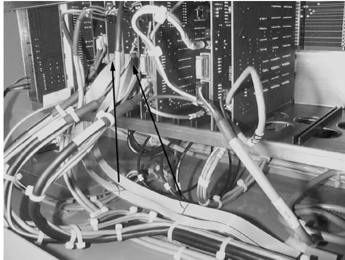
Figure 11-87 Secure Cable to Bottom of Cabinet
