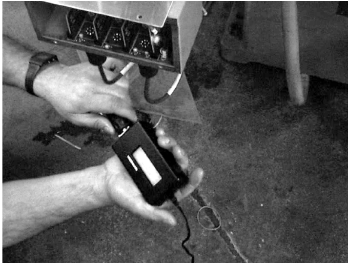
Figure 11-103 Plug Pin Connector Into Scale Test Box
