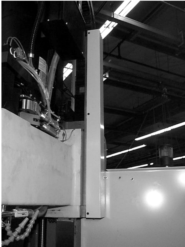
Figure 11-73 Attach Scale Cover to Scale
