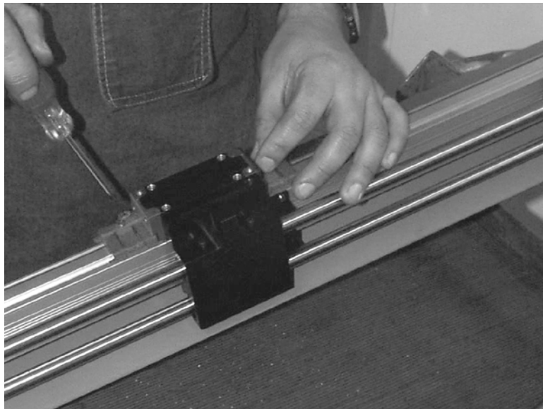
Figure 11-38 Remove Packing Clips from Scale Assembly
