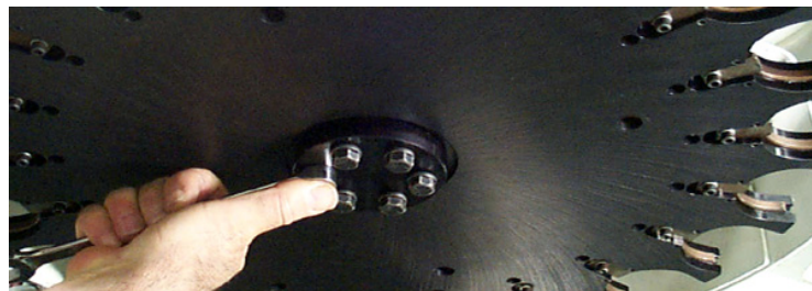
Figure 5-6 Loosen Hex Bolts Holding Tool Carrier
