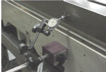
Figure 6-12 Set Zero Reading
