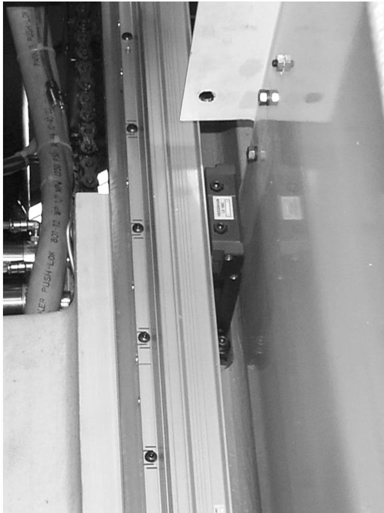
Figure 11-71 Attach Scale Reader to Mounting Bracket
