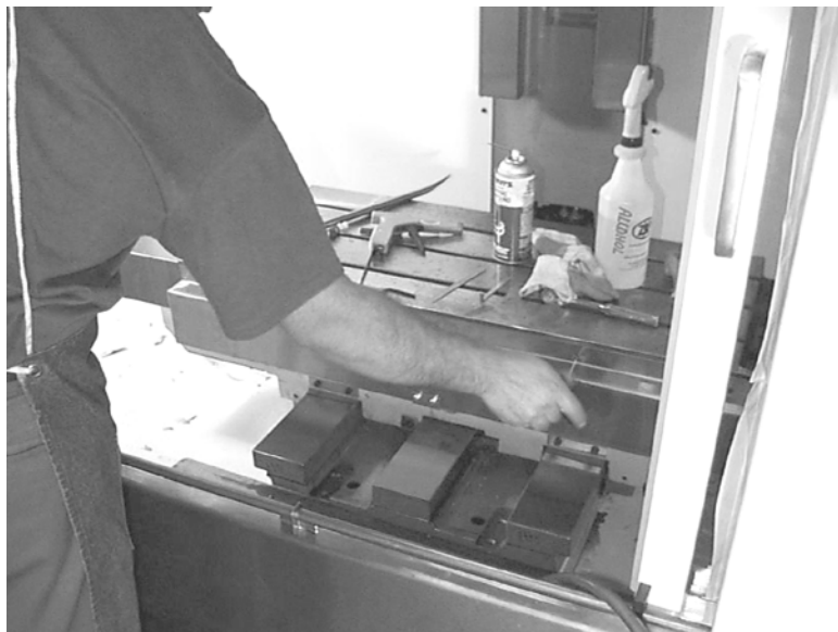
Figure 11-30 Attach Axis Position Indicator to Scale Cover
