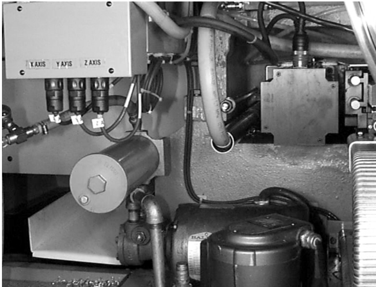
Figure 11-57 Route Cables to Back of Control Cabinet
