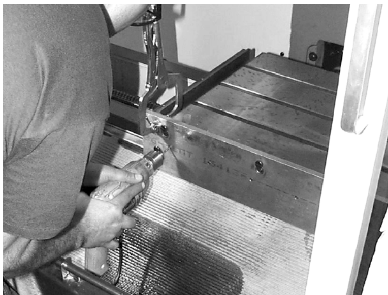
Figure 11-7 Drill Starting Holes
