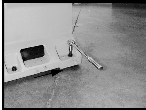
Figure 3-19 Drive Down Corner Leveling Screws
