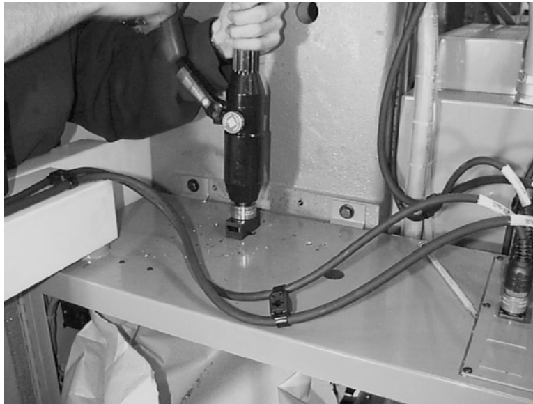
Figure 11-95 Create Opening for Fourth Axis Ribbon Cable
