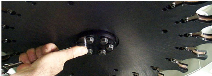
Figure 5-7 Loosen Hex Bolts on Under Side of Tool Carrier
