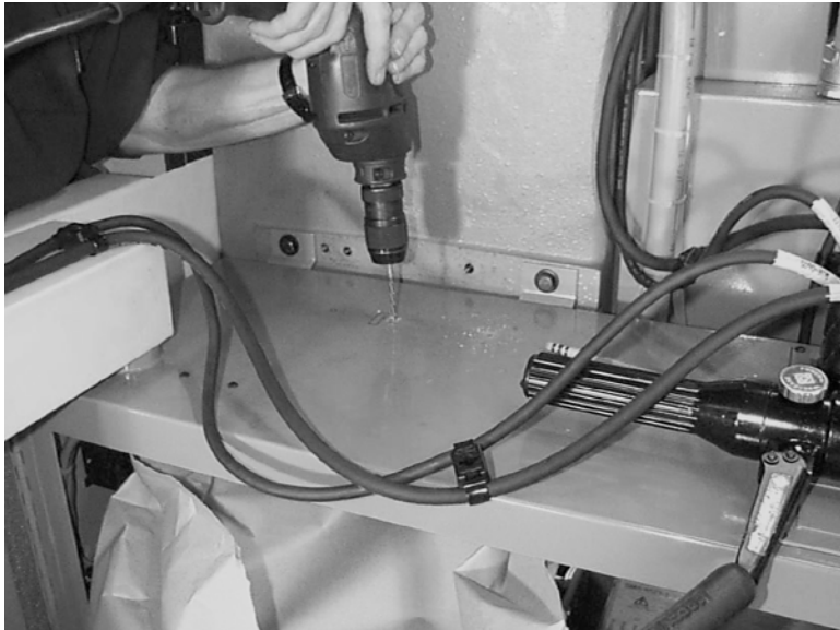
Figure 11-93 Drill Starting Holes
