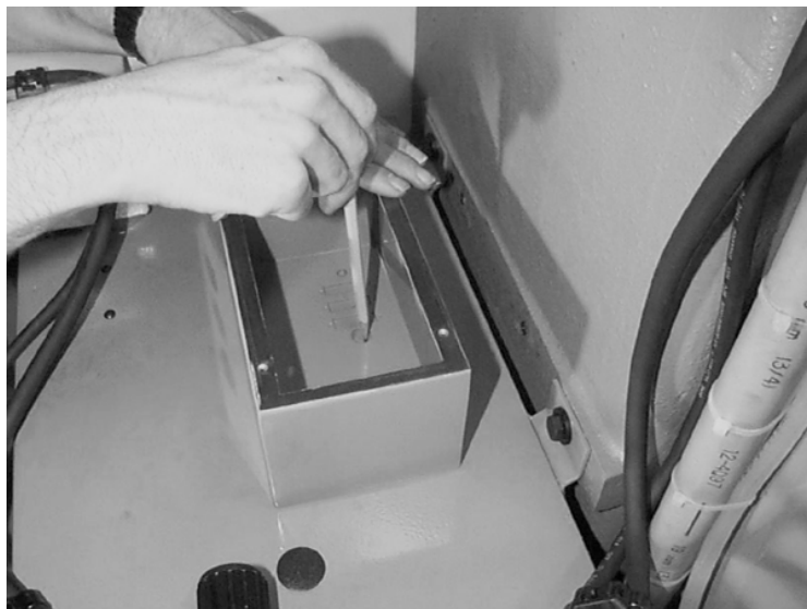
Figure 11-90 Mark Positions to be Drilled Out
