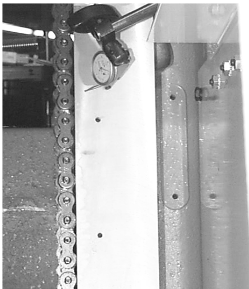
Figure 11-61 Mount Dial Indicator to Column
