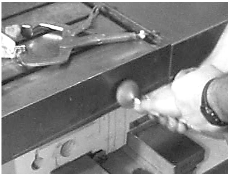
Figure 11-11 Clean Debris from Holes
