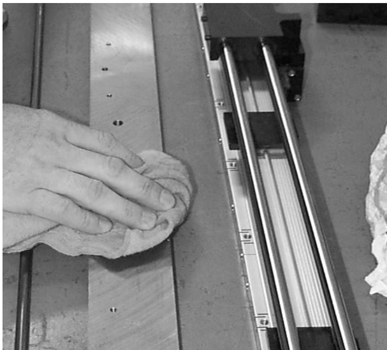
Figure 11-63 Thoroughly Clean Z Axis Mounting Plate
