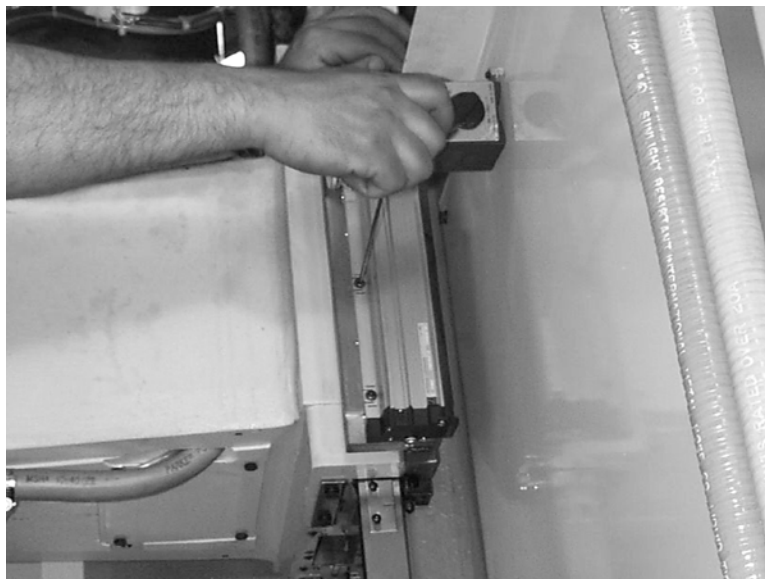
Figure 11-68 Attach Scale to Mounting Plate
