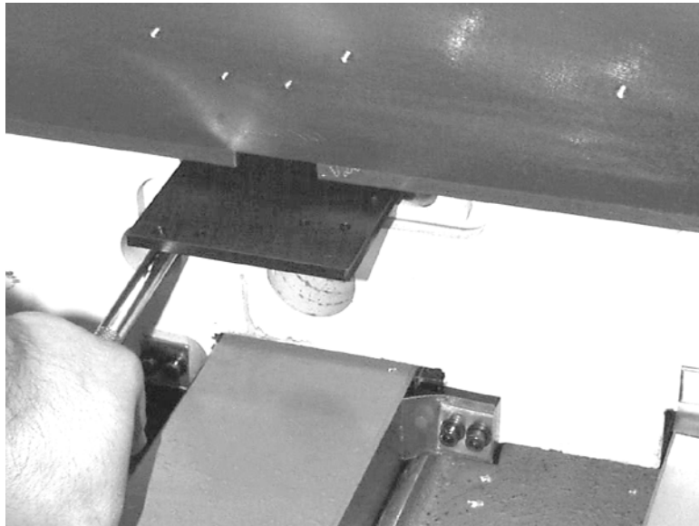
Figure 11-17 Install X Axis Scale Reader Mounting Screws
