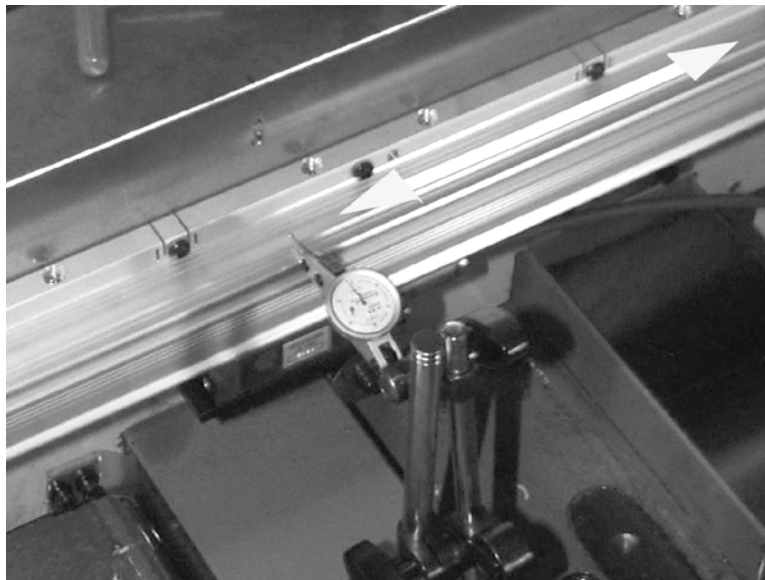
Figure 11-24 Mount Scale to Table
