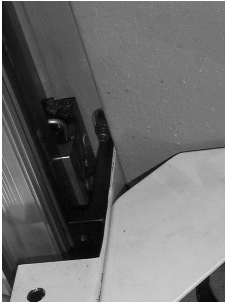
Figure 11-70 Attach Z Axis Mounting Bracket to Column
