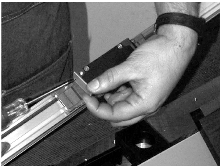
Figure 11-19 Remove Protective Cover from Pin Connector
