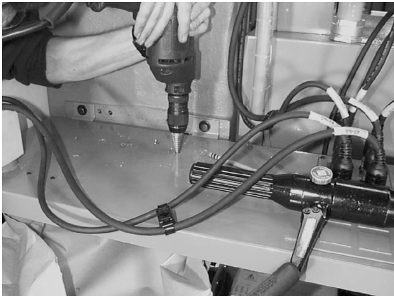
Figure 11-94 Open Holes with Step Drill
